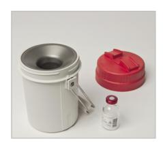
The shielded container is a certified type A container, made of lead or tungsten. The container can be used in combination with the outer case for safe transport of vials containing radioactive substances by road or air. The cylindrical body and top are made of lead or tungsten and the interior has a plastic insert and is slightly cone shaped for easy loading of the vials. The insert is suitable for different injector systems including the KARL100.
